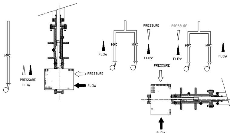
Special care should be taken to maintain the correct distance between the flanges and to ensure that they are parallel to the valve body. Incorrect alignment of the valve can cause deformations, which can lead to difficulties in operation.
