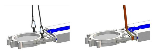
Fig. 1 Handling with eyebolts
